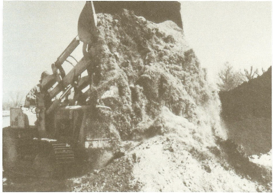
Finished compost is mixed with sand and topsoil for use on athletic fields.
